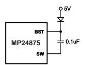
Figure 2—External Bootstrap Diode
