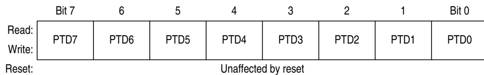
Figure 11-13. Port D Data Register (PTD)
