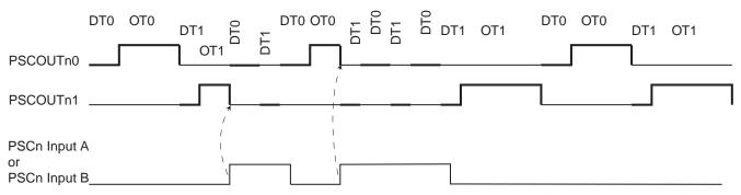
Used in Fault mode 5, PSCn Input A or PSCn Input B act indifferently on On-Time0/Dead-Time0 or on On-Time1/Dead-Time1.
