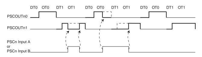
Figure 15-26. PSC behaviour versus PSCn Input A or Input B in Mode 4
