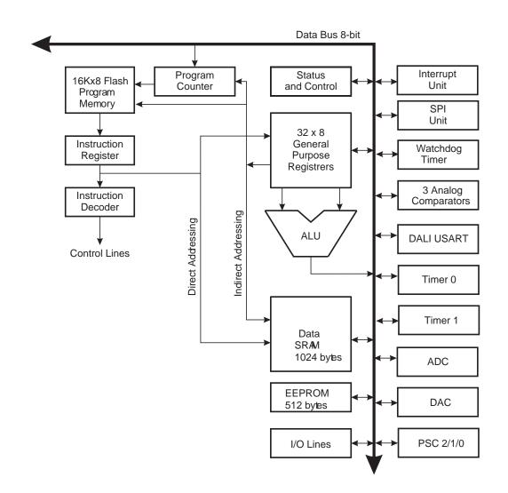
The AVR core combines a rich instruction set with 32 general purpose working registers. All the 32 registers are directly connected to the Arithmetic Logic Unit (ALU), allowing two independent registers to be accessed in one single instruction executed in one clock cycle. The resulting architecture is more code efficient while achieving throughputs up to ten times faster than conventional CISC microcontrollers.
