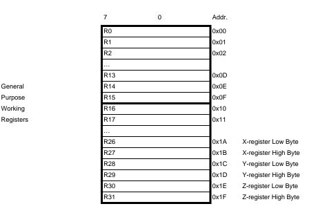
Figure 4-2. AVR CPU General Purpose Working Registers
