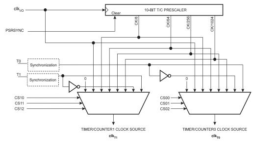
Figure 12-2. Prescaler for Timer/Counter0 and Timer/Counter1<sup>(1)</sup>
