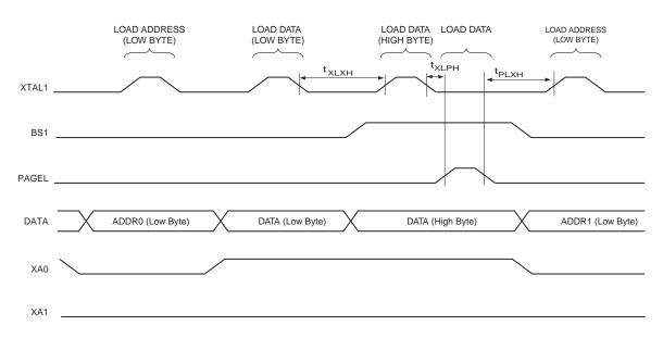
Note: 1. The timing requirements shown in Figure 25-5 (i.e.,  $t_{DVXH}$ ,  $t_{XHXL}$ , and  $t_{XLDX}$ ) also apply to loading operation.
