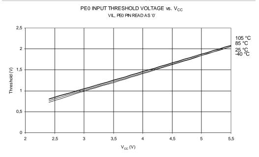
Figure 26-29. PE0 Input Threshold Voltage vs. V<sub>CC</sub> (PE0 Pin Read As '0')
