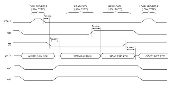
Note: 1. The timing requirements shown in Figure 25-5 (i.e.,  $t_{DVXH}$ ,  $t_{XHXL}$ , and  $t_{XLDX}$ ) also apply to reading operation.
