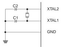
The Oscillator can operate in three different modes, each optimized for a specific frequency range. The operating mode is selected by the fuses CKSEL3..1 as shown in Table 6-3.
