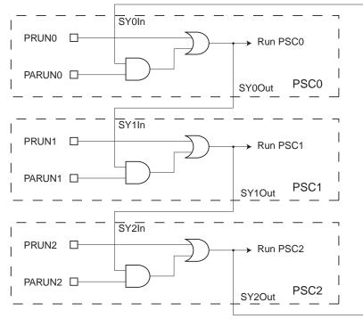
Figure 15-38. PSC Run Synchronization
