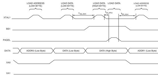
Note: 1. The timing requirements shown in Figure 24-7 (i.e., t<sub>DVXH</sub>, t<sub>XHXL</sub>, and t<sub>XLDX</sub>) also apply to loading operation.
