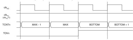
Figure 13-8. Timer/Counter Timing Diagram, no Prescaling
