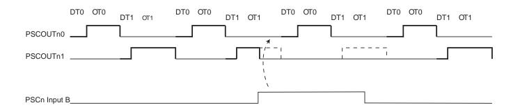
The output is disactivated while retriggering input is active.
