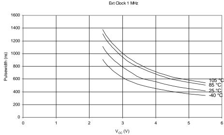
RESET PULSE WIDTH vs. V<sub>CC</sub> Ext Clock 1 MHz
