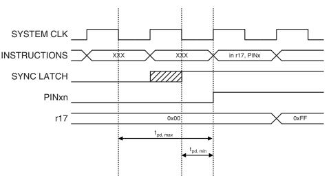
Consider the clock period starting shortly after the first falling edge of the system clock. The latch is closed when the clock is low, and goes transparent when the clock is high, as indicated by the shaded region of the "SYNC LATCH" signal. The signal value is latched when the system clock goes low. It is clocked into the PINxn Register at
