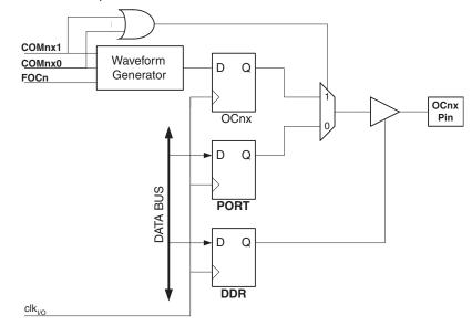
Figure 13-4. Compare Match Output Unit, Schematic
