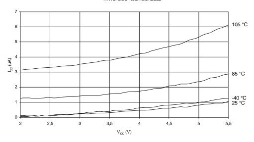
Figure 26-9. Power-Down Supply Current vs. V<sub>CC</sub> (Watchdog Timer Disabled) POWER-DOWN SUPPLY CURRENT vs. V<sub>CC</sub> WATCHDOG TIMER DISABLED
