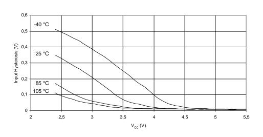
RESET PIN INPUT HYSTERESIS vs.  $V_{\text{CC}}$
