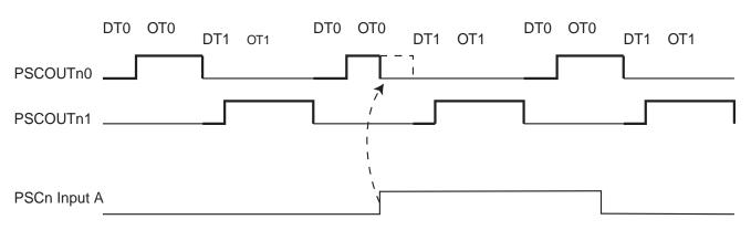
Figure 15-33. PSC behaviour versus PSCn Input A in Mode 9
