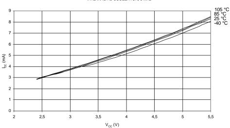
ACTIVE SUPPLY CURRENT vs. V<sub>CC</sub> INTERNAL RC OSCILLATOR, 8 MHz
