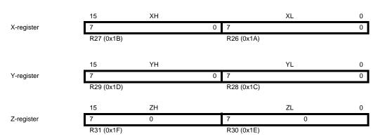
Figure 4-3. The X-, Y-, and Z-registers
