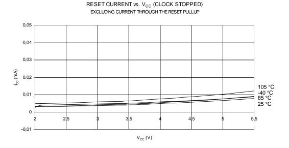
Figure 26-47. Reset Supply Current vs. V<sub>CC</sub> (Clock Stopped, Excluding Current through the Reset Pull-up)
