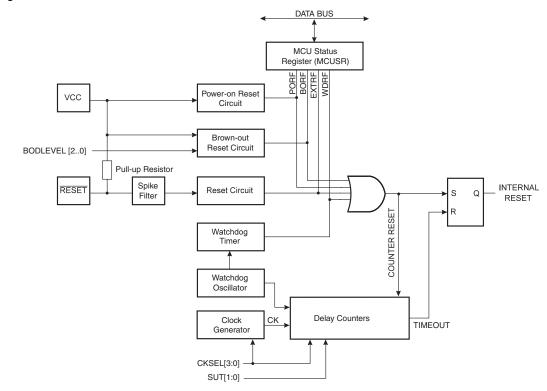
Figure 8-1. Reset Logic
