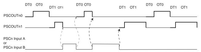
Figure 15-29. PSC behaviour versus PSCn Input A in Fault Mode 6
