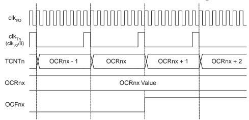
Figure 14-12 shows the count sequence close to TOP in various modes. When using phase and frequency correct PWM mode the OCRnx Register is updated at BOTTOM. The timing diagrams will be the same, but TOP should be replaced by BOTTOM, TOP-1 by BOTTOM+1 and so on. The same renaming applies for modes that set the TOVn Flag at BOTTOM.
