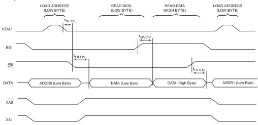
Note: 1. The timing requirements shown in Figure 24-7 (i.e.,  $t_{DVXH}$ ,  $t_{XHXL}$ , and  $t_{XLDX}$ ) also apply to reading operation.
