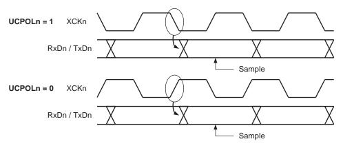
The UCPOL bit UCRSnC selects which XCK clock edge is used for data sampling and which is used for data change. As Figure 17-3 shows, when UCPOL is zero the data will be changed at rising XCK edge and sampled at falling XCK edge. If UCPOL is set, the data will be changed at falling XCK edge and sampled at rising XCK edge.
