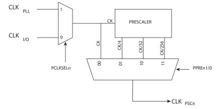
PCLKSELn bit in PSC n Configuration register (PCNFn) is used to select the clock source.
