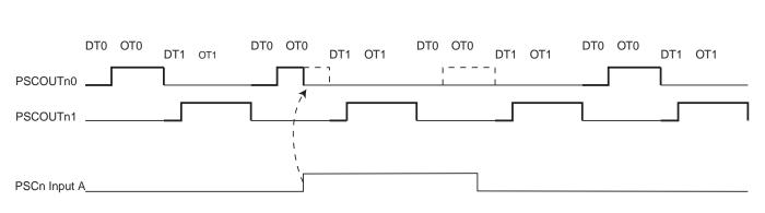
Figure 15-35. PSC behaviour versus PSCn Input A in Mode 14
