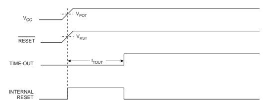
Figure 8-3. MCU Start-up, RESET Extended Externally
