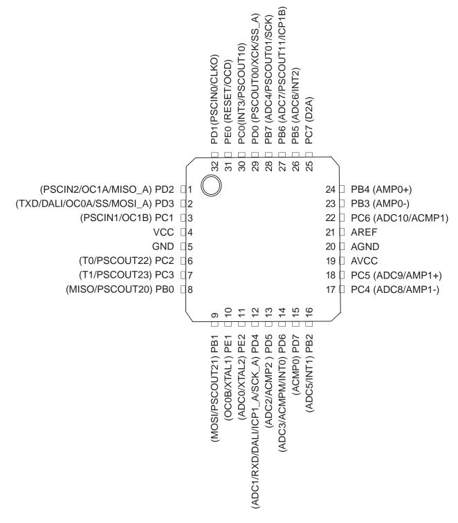
Note: The Center GND PADDLE has to be connected to GND.
