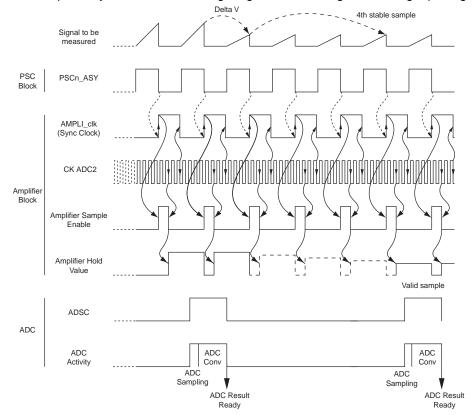
Figure 20-15. Amplifier synchronization timing diagram with change on analog input signal.
