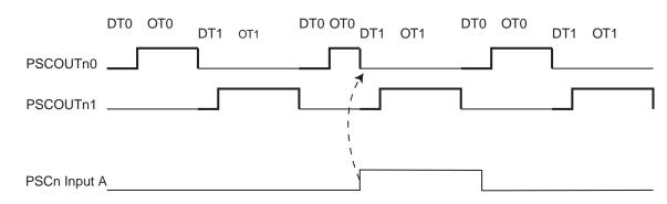
Figure 15-31. PSC behaviour versus PSCn Input A in Mode 8
