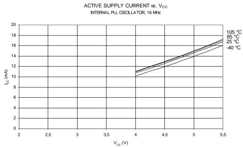
Figure 26-4. Active Supply Current vs. V<sub>CC</sub> (Internal PLL Oscillator, 16 MHz)
