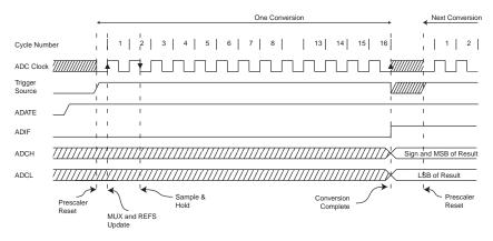
Figure 20-7. ADC Timing Diagram, Free Running Conversion
