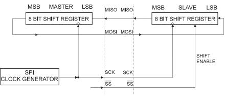
Figure 16-2. SPI Master-slave Interconnection
