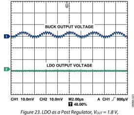
Figure 23. LDO as a Post Regulator,  $V_{OUT} = 1.8 V$ , Load Current = 500 mA,  $V_{OUT2} = 1.2 V$ , Load Current = 50 mA
