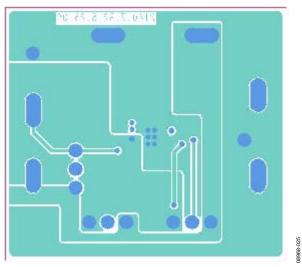
Figure 25. Typical Board Layout, Bottom Side
