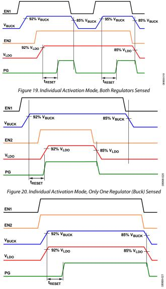
Figure 21. Individual Activation Mode, No Activation/Deactivation Delay Between Regulators, EN1 and EN2 Pins Tied Together
