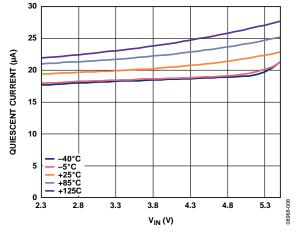
Figure 9. Quiescent Current vs. Input Voltage
