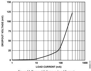
Figure 13. Dropout Voltage vs. Load Current
