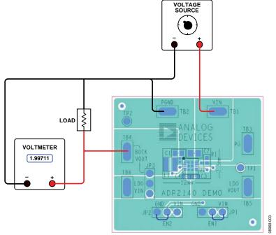
Figure 3. Buck Output Voltage Regulation Measurement Setup
