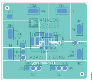
Figure 24. Typical Board Layout, Top Side
