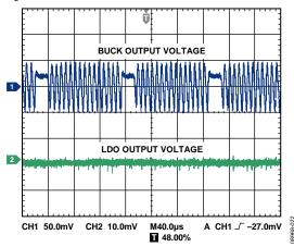
Figure 22. LDO as a Post Regulator,  $V_{OUT} = 1.8$  V, Load Current = 50 mA,  $V_{OUT2} = 1.2$  V, Load Current = 50 mA
