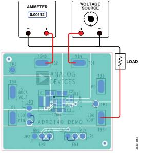
Figure 14. LDO Ground Current Measurement
