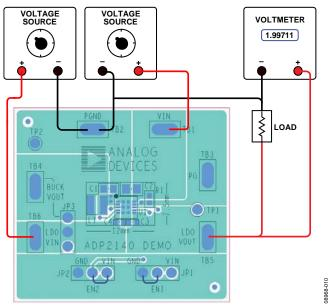
Figure 10. LDO Output Voltage Regulation Measurement Setup
