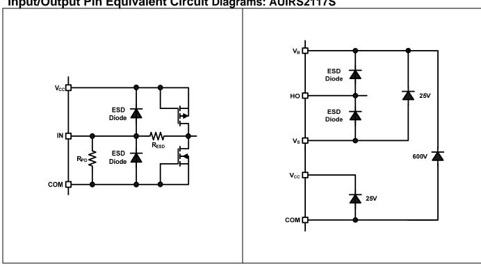
Input/Output Pin Equivalent Circuit Diagrams: AUIRS2118S
