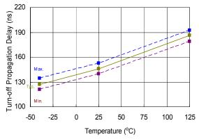
Figure 15. Turn-Off Time vs. Temperature
