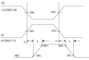
Figure 4: Switching Time Waveform Definition
