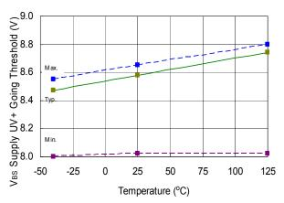
Figure 27. V<sub>BS</sub> Undervoltage Threshold (+) vs. Temperature
