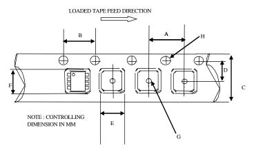
CARRIER TAPE DIMENSION FOR 8SOICN
