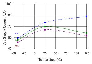
Figure 21. V<sub>BS</sub> Supply Current vs. Temperature
