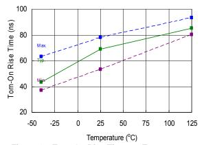
Figure 16. Turn-On Rise Time vs. Temperature
