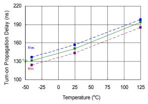
Figure 14. Turn-On Time vs. Temperature
