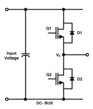
Figure 5: Half Bridge Circuit
