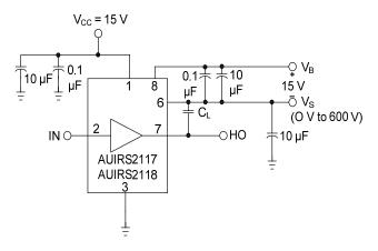
Figure 3: Switching Time Test Circuit
