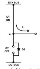
Figure 6: Q1 conducting
