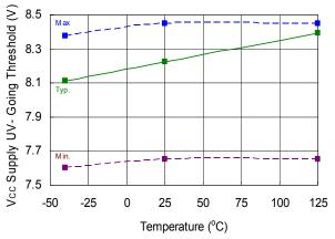
Figure 26. V<sub>CC</sub> Undervoltage Threshold (-) vs. Temperature
