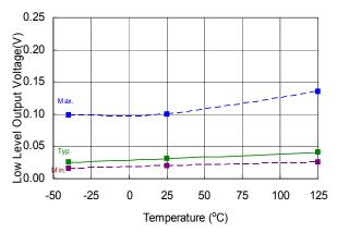
Figure 19. Low Level Output Voltage vs. Temperature
