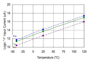
Figure 23. Logic "1" Input Current vs. Temperature
