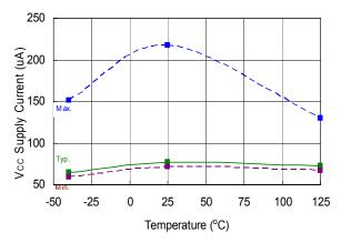
Figure 22. V<sub>CC</sub> Supply Current vs. Temperature
