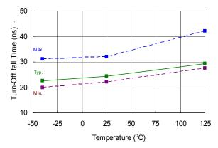
Figure 17. Turn-Off Fall Time vs. Temperature
