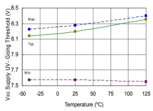
Figure 28. V<sub>BS</sub> Undervoltage Threshold (-) vs. Temperature
