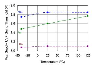
Figure 25. V<sub>CC</sub> Undervoltage Threshold (+) vs. Temperature
