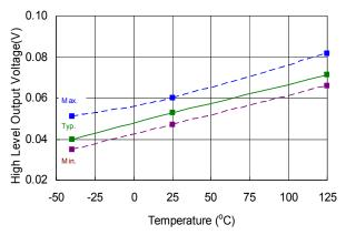
Figure 18. High Level Output Voltage vs. Temperature
