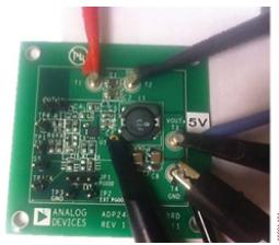
Figure 4. Switch Node Measurement
