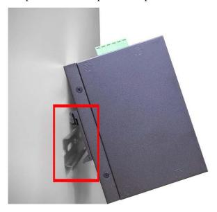
4. Then, lightly push the bottom of the switch so it can snap the rest of the way onto the DIN rail track.
